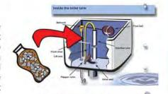
water per flush. New systems only require 6 litres of water
