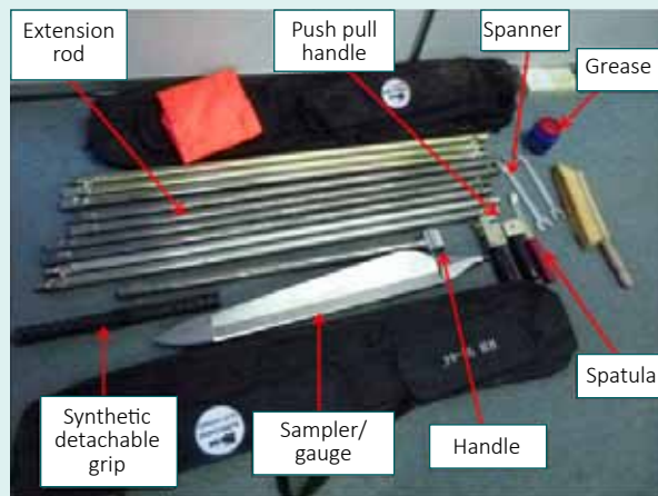
Figure 1.2: Peat auger tools and method to use this auger (Credit: Global Environment Centre, GEC)
