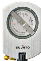
Figure 8: Clinometer. Measures the height of trees.
