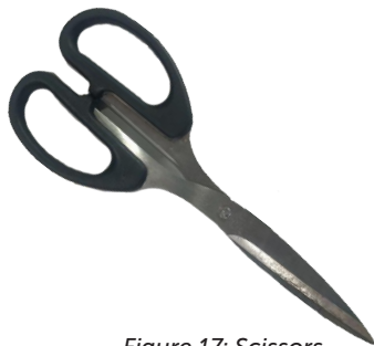
Figure 17: Scissors. Cuts thinner material.
