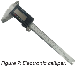
Figure 7: Electronic calliper. Measures the diameter of trees with high accuracy.
